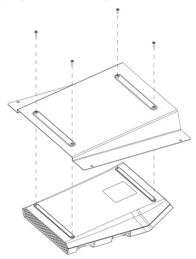
3. Offer up the DL1608 to the rack and secure it in place with four rack screws (not supplied). Be sure to use the PadLock included with your DL1608 to ensure that the iPad stays safe and secure during transport with the mixer. Also, remember to leave enough room at the top of the rack to attach the DC power cord and any other connections needed.
