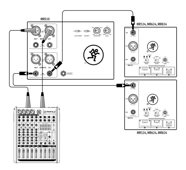
Connecting an MRS10 to the signal chain is quite easy, so let's take a quick look at a fairly typical setup. In this example, whatever sources you desire are plugged into the mixer's inputs. [Note: you could also plug a source – such as a smartphone or other mp3 player – directly into the subwoofer's input(s)].
