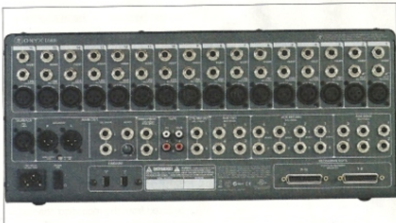
All ins and outs – and there are plenty of them – are housed on the FlexiPod, a separate unit which can be mounted behind or on top of the main body or separately in a standard 19-inch rack.
