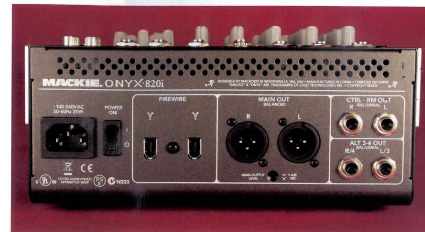
The rear of the Onyx 820i is home to the unit's two Firewire sockets, XLR duplicates of the main outputs and the Control Room and Alt outputs.
